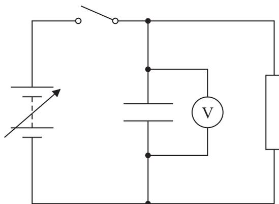
The potential difference (p.d.)  $V$  across the capacitor decreased as the capacitor discharged. The technician measured values of  $V$  at corresponding times  $t$  until the p.d. was half its initial value.
